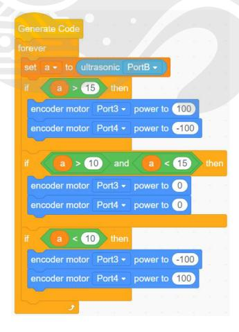
Note: The RGB ultrasonic sensor detected value, which can make robot stop moving, must be an interval. Because RGB ultrasonic sensor detected value will wave, if it is not a range but a specific value, the robot will move back and forward instead of being static.
